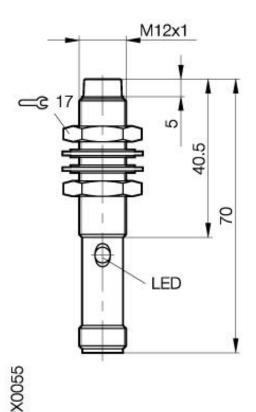
Inductive Sensors BES 516-544-S 4-H M12x1 x 70 normally-open Sn=4mm unshielded
